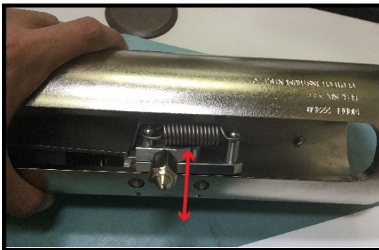
Push arm in to test compression springs
